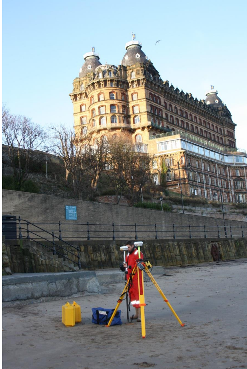
Figure 10. Trimble R4 GNSS RTK base and rover system used for positioning during the study.
