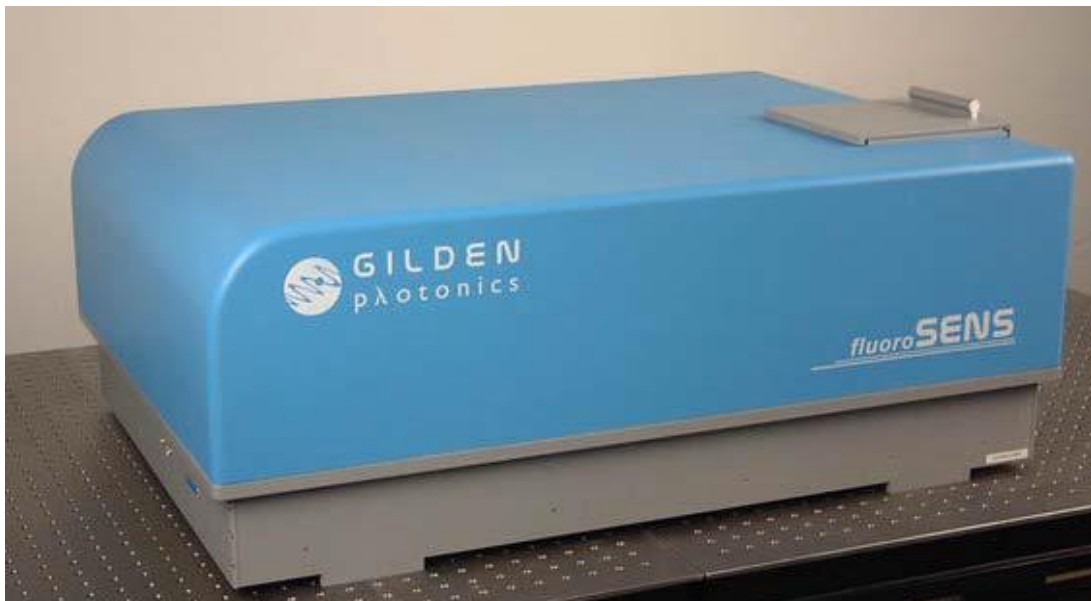
Figure 11. The Fluorosens laboratory fluorimeter.
